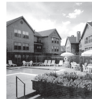
Fig. 3 - Use building masses to frame and enclose formal open space. Notice how the buildings define the outdoor patio area.
