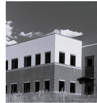
Fig. 1 - Create a distinguishable building base, middle, and cap. Notice how the base creates a pedestal for the building to rest upon, while belly bands distinguish individual floors.
