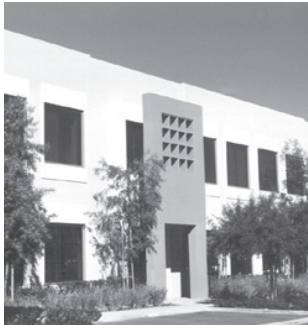
Fig. 8 - Layer building planes to increase façade variety and visual interest, creating a layered effect that adds rich shadow patterns.
