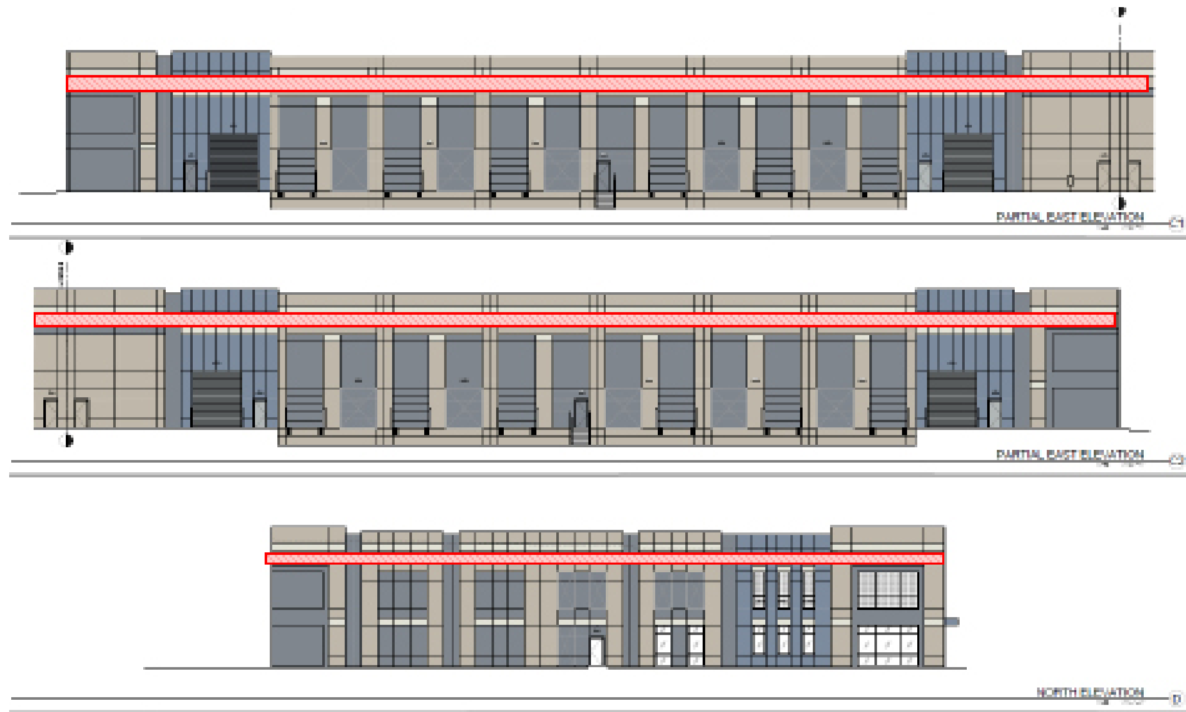
Figure 20.A - Wall Mounted Sign Location Options
