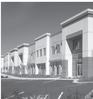
Fig. 10 - Use building projections to increase facade variety and visual interest. Notice how the building projections coupled with the cornice elements create ample facade articulation.
