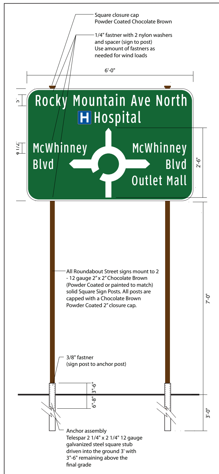
fig. 18e Roundabout Directional Signs
