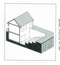
FIGURE 4.1 Excavated walkouts similar to the one illustrated here shall not be permitted.
